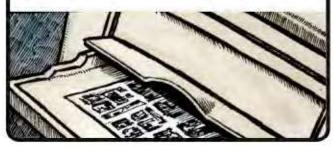
6. Print "master copy two" onto the flip side of the press sheet—making eight page images on the front, and eight on the back.
