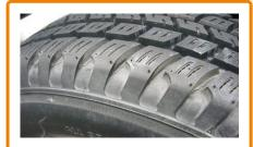
Car tires are made out of rubber with patterned treads. This helps the car grip the road better so it does not slide when turning.
